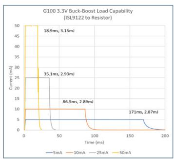
Data provided is by actuation using mechanical cycle tester as reference. Higher current and shorter duration loads lose less energy to quiescent currents and idle loads and operate closer to peak efficiency.
